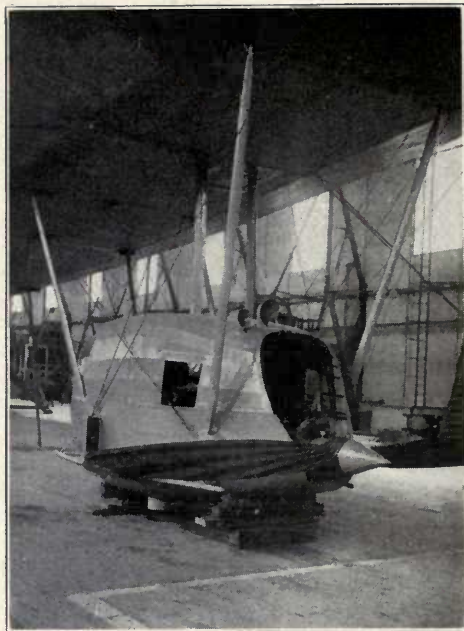
The "DELAG" Passenger Zeppelin "Bodensee." Front and rear views of rear power gondola. Note radiator temperature control and ladder.
